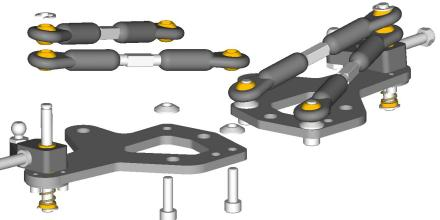
Using the spacers included in the kit, attach the front lower arms to the chassis using the (6) 8-32 flat head phillips screws. Use a full sized screw driver with a tip in good condition. Use of a power screwdriver is not recommended.
