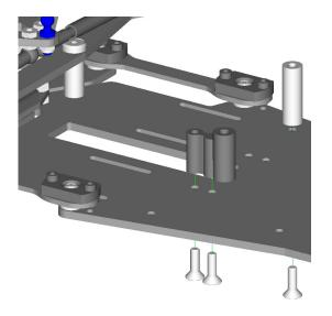
Using the flat head screws, attach the shock/antenna mount, and the stand-off as shown.
