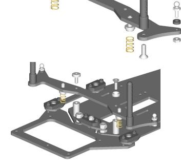
The aluminum bulkheads attach to the lower plate, then the rear plate to the bulkheads, all using flat head screws.
