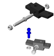
Push straight knurled side of front axle through the knuckle. Be sure to note direction of the knuckle. Use a thin flat nut to secure axle to knuckle.
