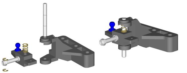
Attach front body mounts as shown using flat head screws.
