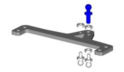
Pre-assemble the top plate with the 2-56 ball studs, then the 4-40 ball stud and spacer. Note orientation in the above drawing. Next attach the top plate with button head screws.
