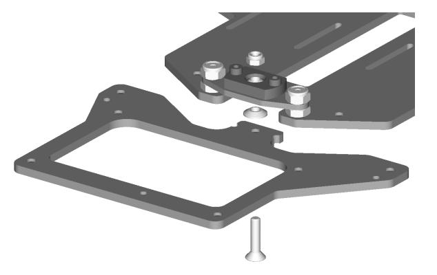
Attach the center pivot to the main chassis, leave the lower nuts loose until the pivot is installed onto the screws. Use needle nose pliers to hold the lower nuts in place while tightening the screws. Then install locking nuts.
