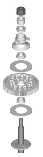
Install bearing carriers into pod plates with flanged bearings. For 12<sup>th</sup> scale, the bearings go toward the bottom. Be sure that you are using the same height axle spacers on each side.
