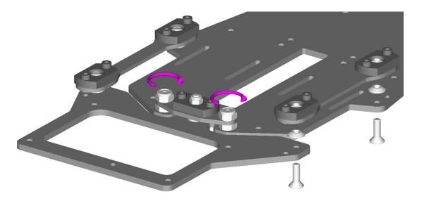
Assemble side links as shown above. Do not over-tighten the 2-56 button head screws. Find a 4-40 screw from the kit, and partially screw it into the ball. Use this screw to judge how much to tighten the 2-56 screws. The ball should not have play in the socket, and it should not be overly tight. There are access holes in the chassis to adjust the 2-56 screws as they seat.
