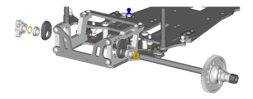
Assemble damper tubes as shown. Only screw the set-screw in half-way.
