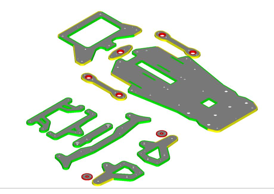
Some people like to sand/seal the chassis and other carbon fiber components with superglue for performance and feel. Do not sand or seal the areas shown highlighted in red. The chassis and rear pod plate areas highlighted in yellow are key areas for measuring the chassis. Care should be taken not to have glue extend below the chassis, as this could affect ride height measurement. Other components highlighted in yellow should not be rounded, only sealed, as this could effect strength.
