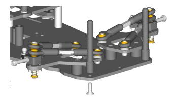
Assemble the caster links first, then the camber links. The notches in the turn buckles should all be on the right side of the chassis. The kit comes with low roll cones under the camber and caster links. Really tighten these screws, they may need to be tightened again.
