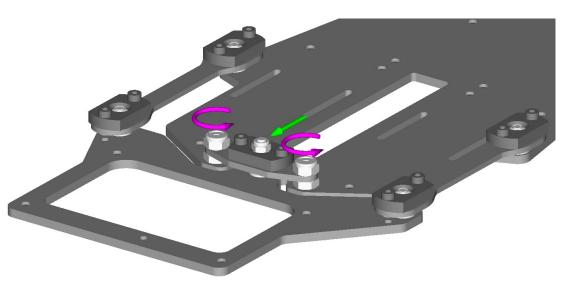
Screw the 6-32 set-screws through the tweak plate so that the wrench side is flush with the top of the tweak plate (the bottom of the tweak plate has counter sunk holes for the body mounts)
