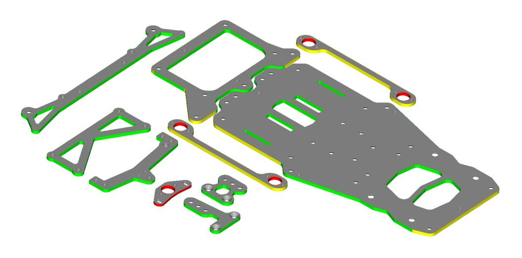
Some people like to sand/seal the chassis and other carbon fiber components with superglue for performance and feel. Do not sand or seal the areas shown highlighted in red. The chassis and rear pod plate areas highlighted in yellow are key areas for measuring the chassis. Care should be taken not to have glue extend below the chassis, as this could affect ride height measurement. Other components highlighted in yellow should not be rounded, only sealed, as this could effect strength.
