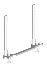
Install the tweak springs, only after the CA glue has fully cured, by pushing and twisting the spring in a clock-wise motion until it 'clicks' into position.
